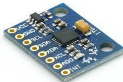
Figure 4.5 MPU-6050 MEMS accelerometer and gyroscope module for vibration sensing
