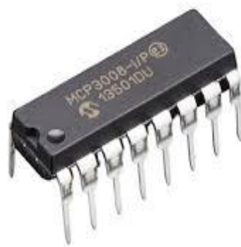
Figure 4.6 MCP3008 ADC interfacing analog sensors with the Raspberry Pi via SPI.
