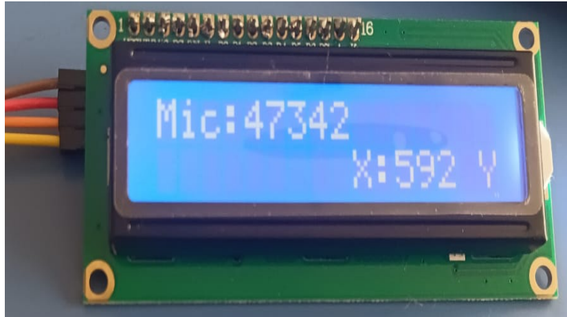
Figure 6.2 LCD Display Showing Real-Time Microphone and Accelerometer Readings
