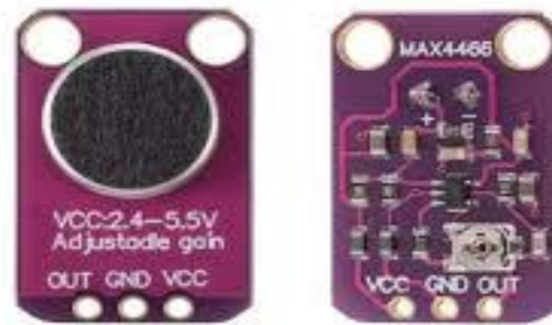
Figure 4.4 High-sensitivity electret condenser microphone with pre-amplifier and band-pass filter
